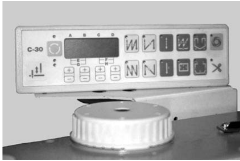
Simple setting for alternating presser foot movement
